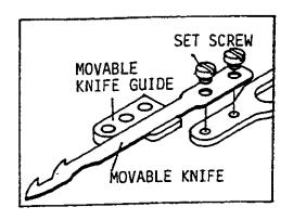
WHEN MOVABLE KNIFE MOVED TO ITS LEFTEST DEAD POINT THERE SHOULD HAVE A INTERVAL OF 1m.m. BETWEEN SET SCREW A AND FIXED KNIFE AND CAN NOT COLLIDE WITH EACH OTHER. YOU CAN ADJUST THE INTERNAL BY LOOSEN THE SET SCREW B AND MAKE SURE THE EDGE OF MOVABLE KNIFE MATCH EVENLY WITH THE EDGE OF FIXED KNIFE.
